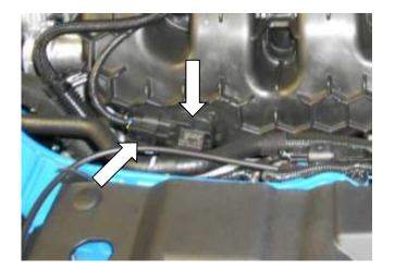
Lift and secure the bonnet and begin by removing the engine cover, this will give better access while carrying out the installation. Disconnect the wiring to the sensor.
